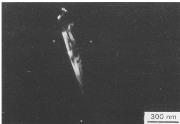
Figure 9 Dark-field image of a rod-like secondary silicon-rich particle after HIPing at 550°C and 68.95 MPa for 120 min.
