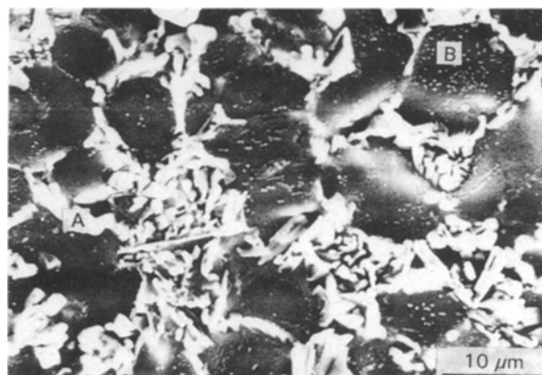
Figure 2 Primary and secondary silicon-rich particles in an aluminium-rich matrix of the as-cast material.
