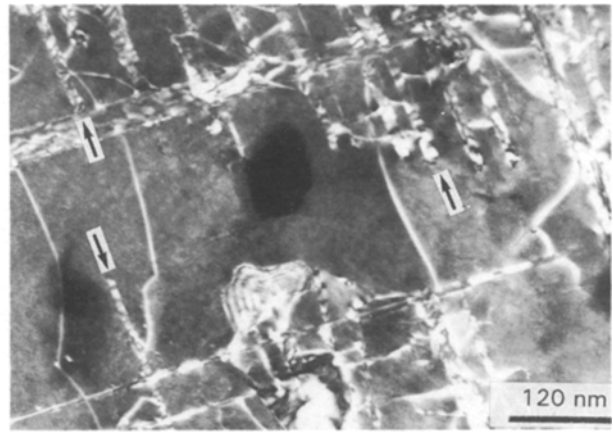
Figure 15 Weak-beam image of iron-containing particles after ageing for 48 h.
